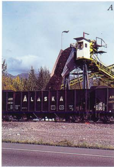
A) Unit trains of gravel hauled 2.6 million tons from the Matanuska- Susitna Valley.
