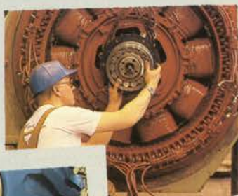
Jim Trueblood, a locomotive electrician in Anchorage, installs a new bearing on a locomotive engine alternator. ▶
