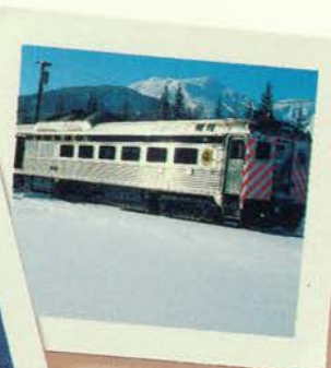
Two self-propelled rail diesel cars, purchased in late 1985, will upgrade passenger service on the Alaska Railroad.
