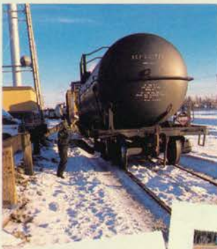
This 20,000-gallon tank car is part of the OWL (Oil Worker Limited), a new, daily unit train that brings jet fuel from North Pole to Anchorage, and returns to Fairbanks with gasoline and other petroleum products.
