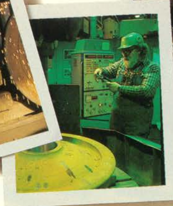
◀ Melvin Hills inspects the assembly of a wheel mounted onto a rail car axle. Hills is a carman in the Fairbanks wheel shop.
