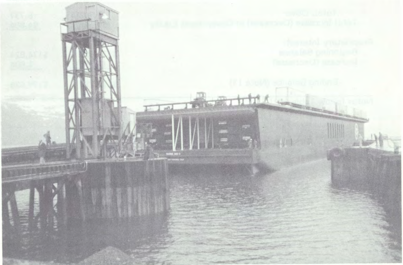
First double-deck barge docks at Railroad's port facility in April 1984. Barge accommodates rail cars on lower level and rubber-tired trailers on upper level. (Photo by Bill Coghill)
