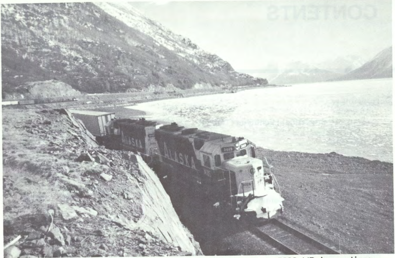
A northbound freight train, powered by two GP-40-2, 3000 HP locomotives, along Turnagain Arm. A record setting 8.3 million tons of freight were moved in FY 1984. (Photo by Bill Coghill)
