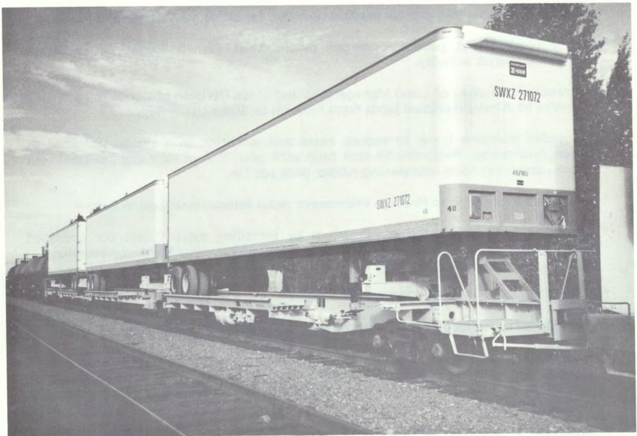
The Railroad started using these articulated intermodal platform cars specifically designed for Alaska TOFC service in 1984. (Photo by Bill Coghill)
